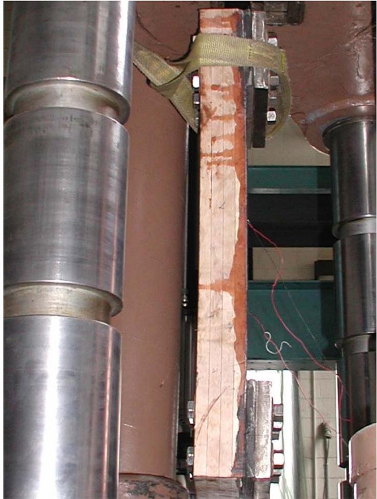
Figure 2: Rail Tension Splice Test
