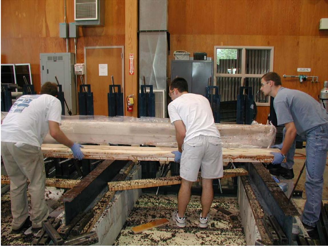
Figure 1: Guardrail Layup in Progress
