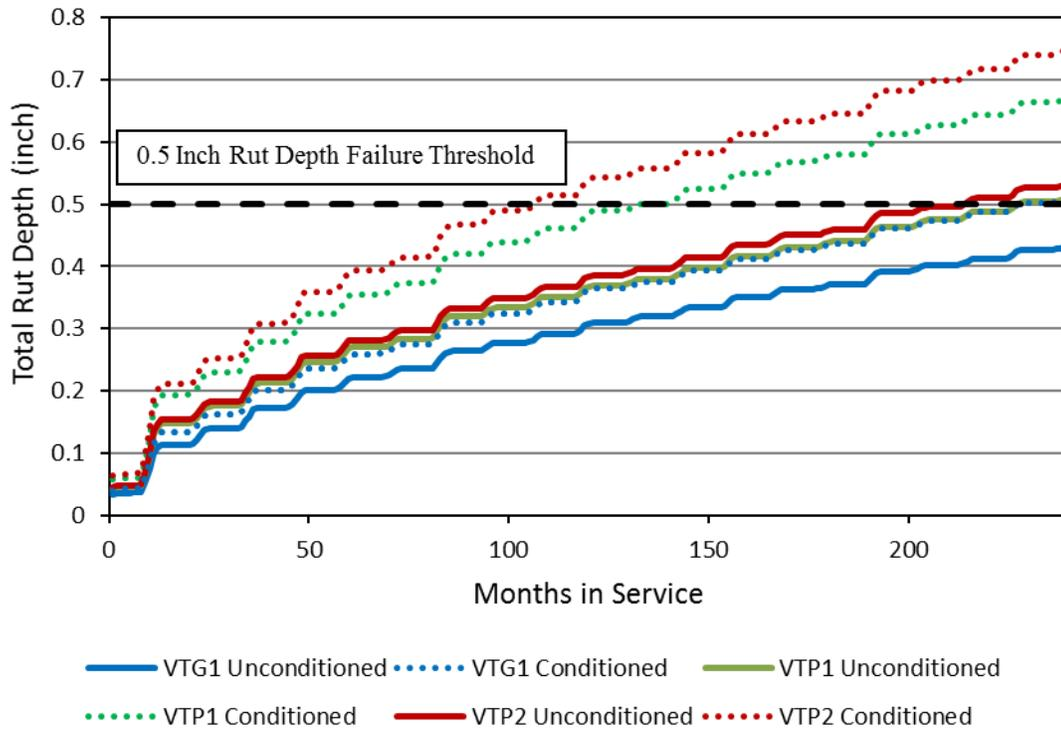
**Figure 1: PavementME Predicted Rut Depth for VT Mixtures**
