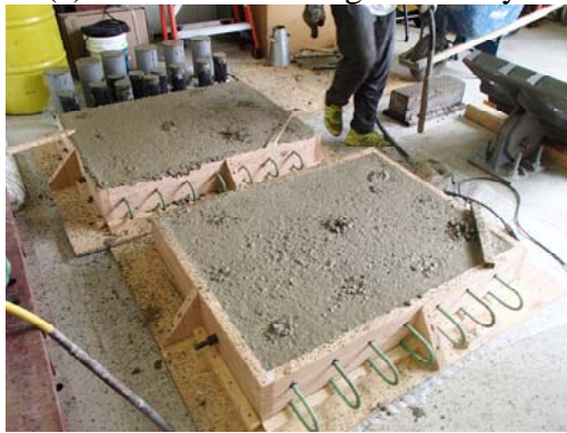
(c) Panels after casting
